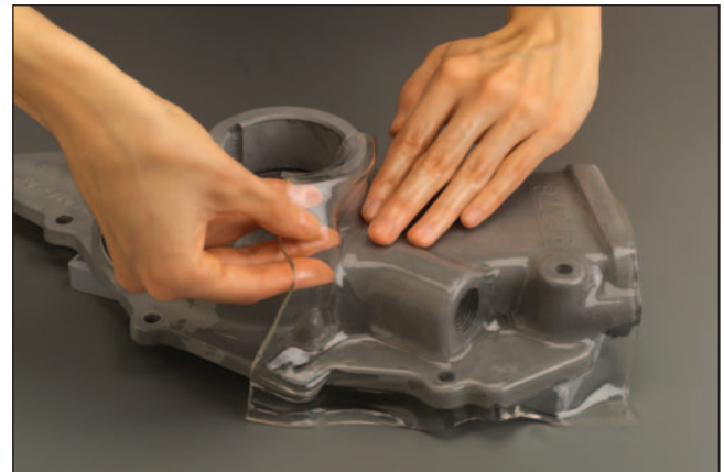
Figure 1. PhotoStress coating being contoured to the surface of a vehicle water pump casting
